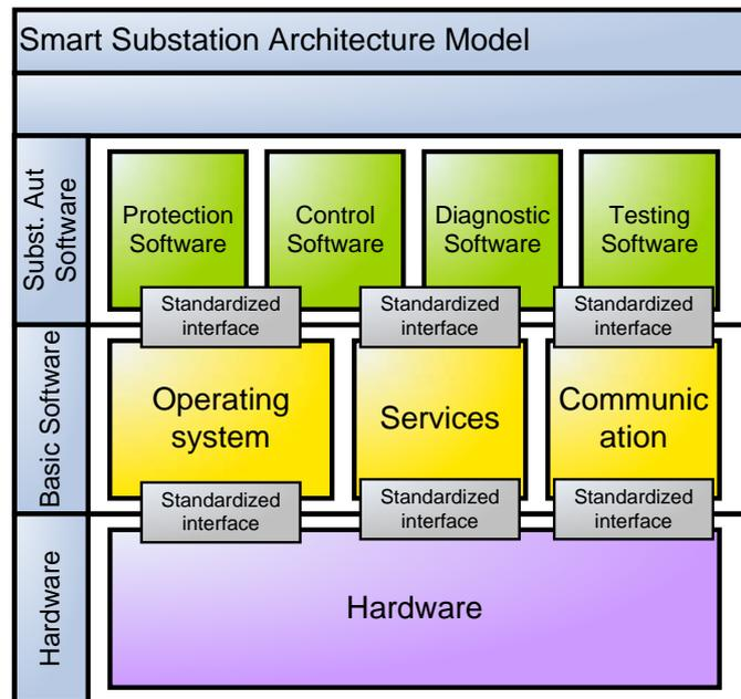
Figure 2. New substation concept [Car10].
