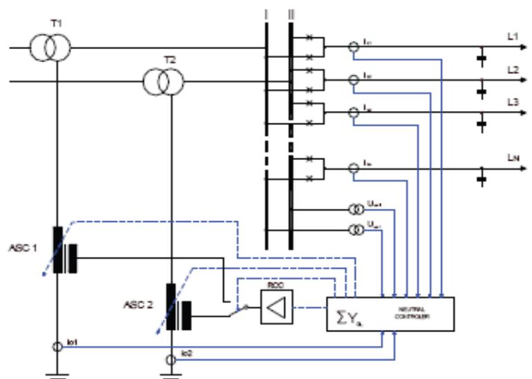
Figure 3. RCC Ground Fault Neutralizer for twin bus bar, block diagram.
