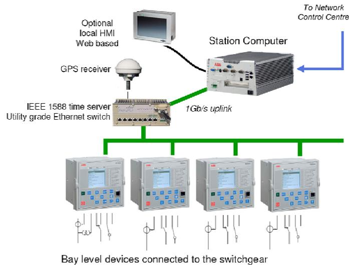
Figure 1. New setup with a central Station Computer [Val09].
