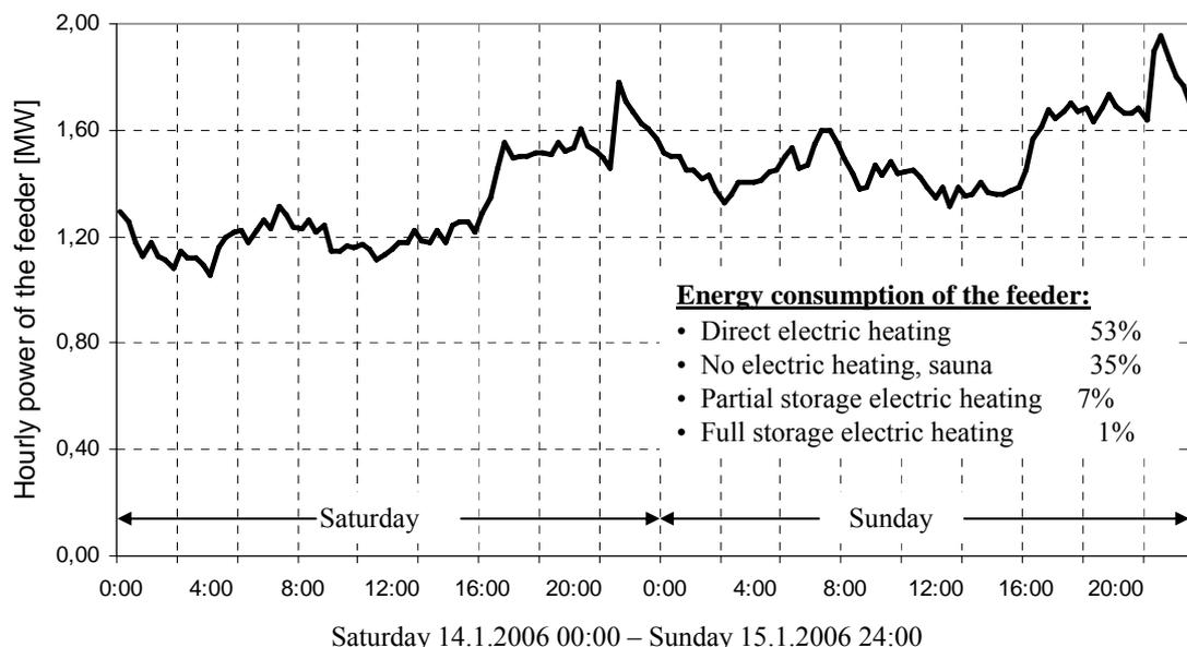
Figure 3. Load curve of the case feeder. Could you change the dates into form 14 Jan 2006?
