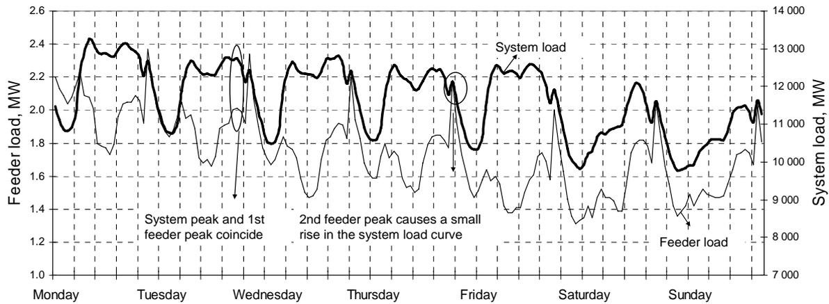
Figure 5. System load and the case feeder load curves.
