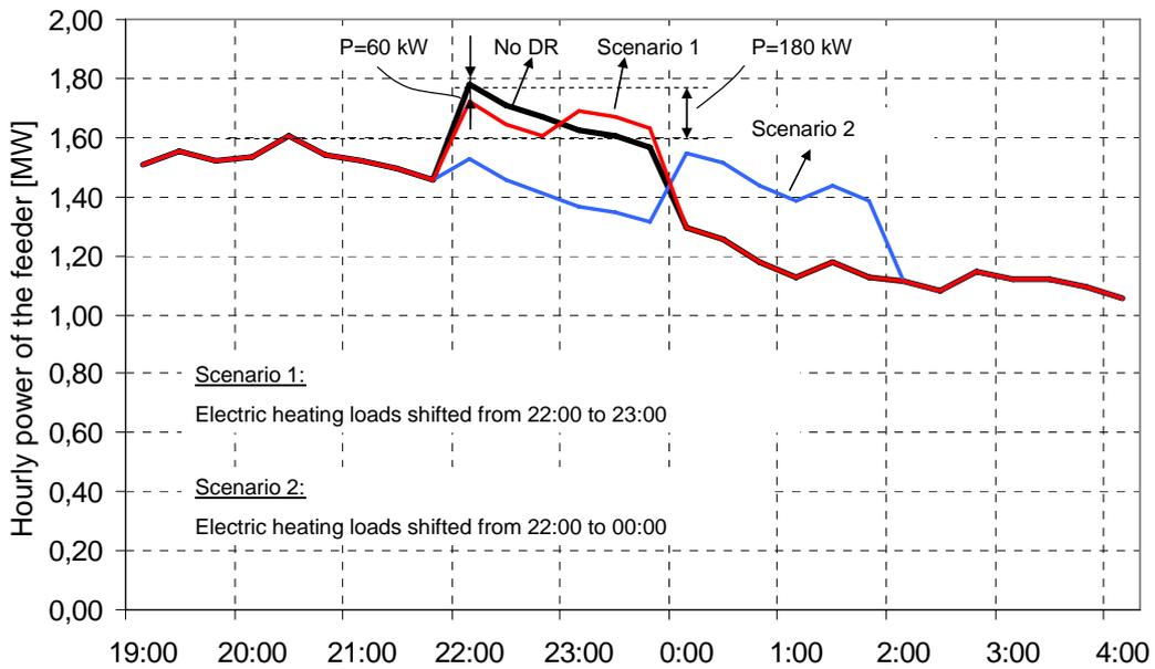
Figure 4. Impact of load control on the load curve. 64 kW is shifted by one hour and 256 kW by two hours.
