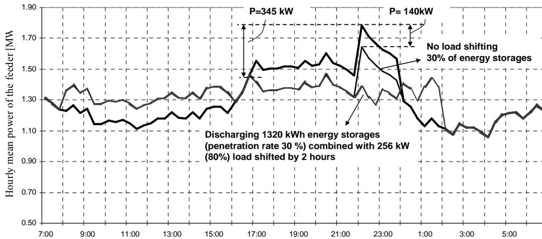
Figure 10. Impact of energy storages on the load curve.
