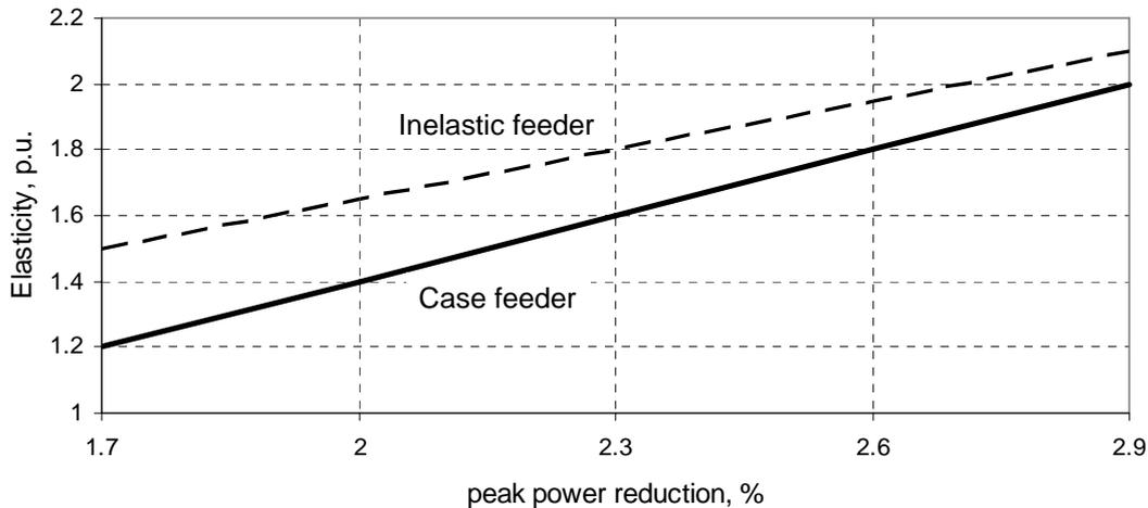
Figure 8. Effect of elasticity on the power peak reduction (no enabling technologies).
