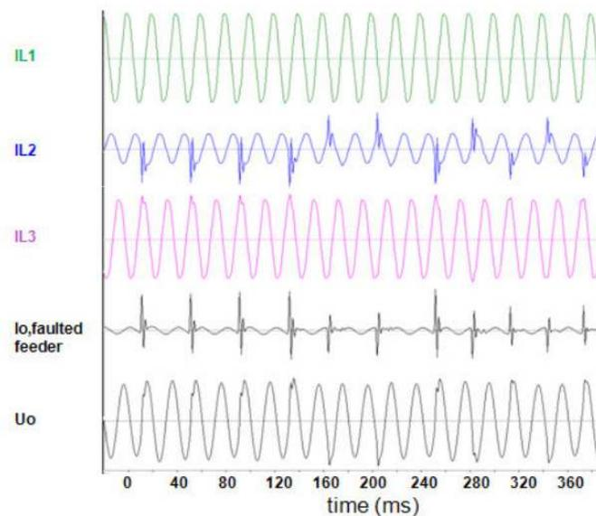
**Figure 5.** Phase currents, zero sequence current at the faulted feeder and neutral point displacement voltage from a real situation, which led to substation disconnection. (Wahlroos 2012.)
