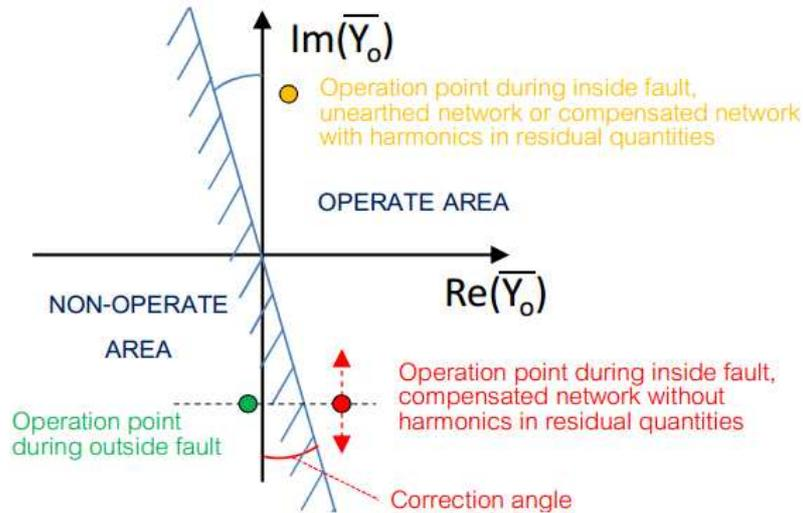
**Figure 13.** Operation characteristic for multi-frequency admittance protection method. (Wahlroos et al. 2013.)
