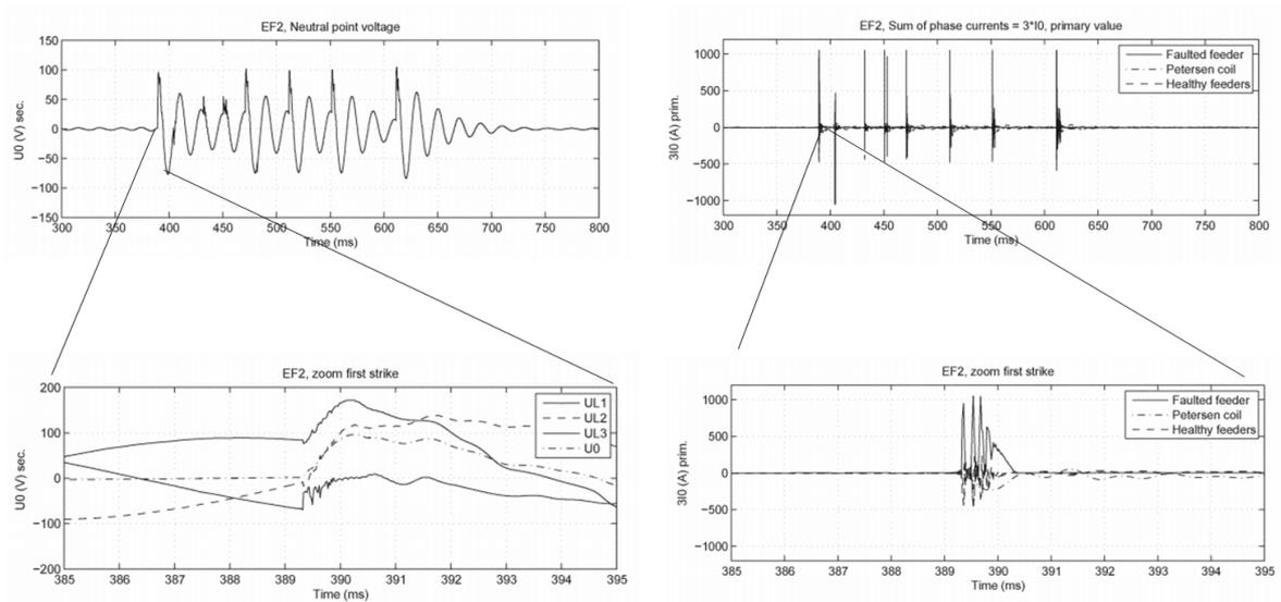
**Figure 6.** Neutral point voltage and sum of phase currents and close-ups in 0.8 second time interval. (Dlaboratory Sweden Ab. 2012.)
