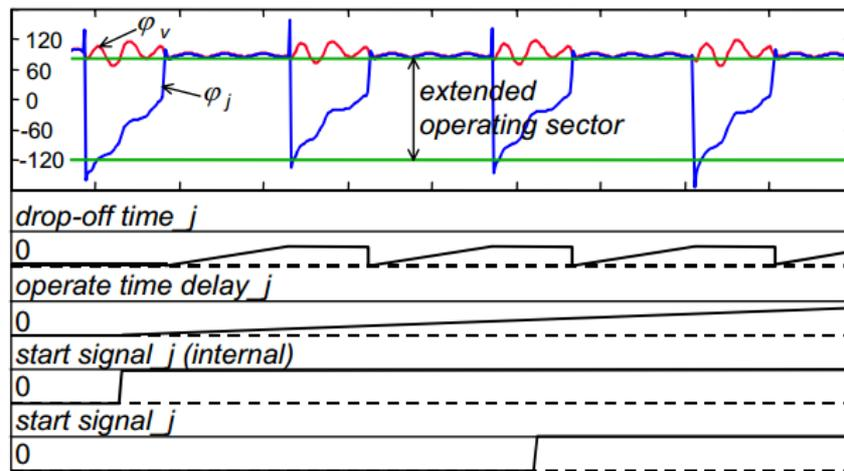
**Figure 9.** Phase angle difference of sampled and filtered residual current and voltage.  $_j$  and  $_v$  means faulty and healthy feeders. (Altonen et al 2003.)
