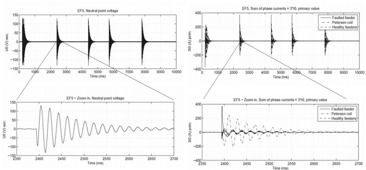
**Figure 3.** Neutral point voltage and sum of phase currents and close-ups in 10 seconds time interval. (Dlaboratory Sweden Ab. 2012.)
