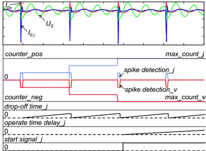
**Figure 8.** Residual currents and voltage of sampled and filtered in scope of spike detection method.  $_j$  and  $_v$  means faulty and healthy feeders. (Altonen et al 2003.)
