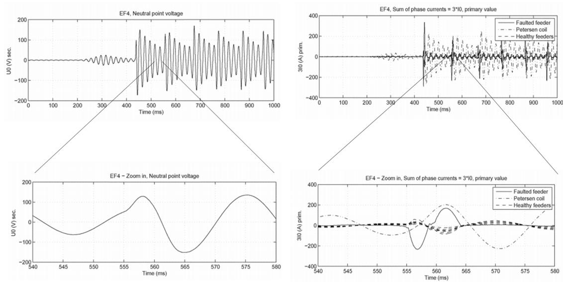
**Figure 4.** Neutral point displacement voltage, residual current, and close-ups in 1 second time interval. (Dlaboratory Sweden Ab. 2012.)
