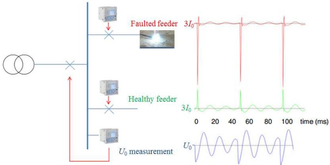
**Figure 1.** Residual currents of faulted and healthy feeders and neutral point displacement voltage waveform in intermittent earth fault situation. (Wahlroos 2012.)
