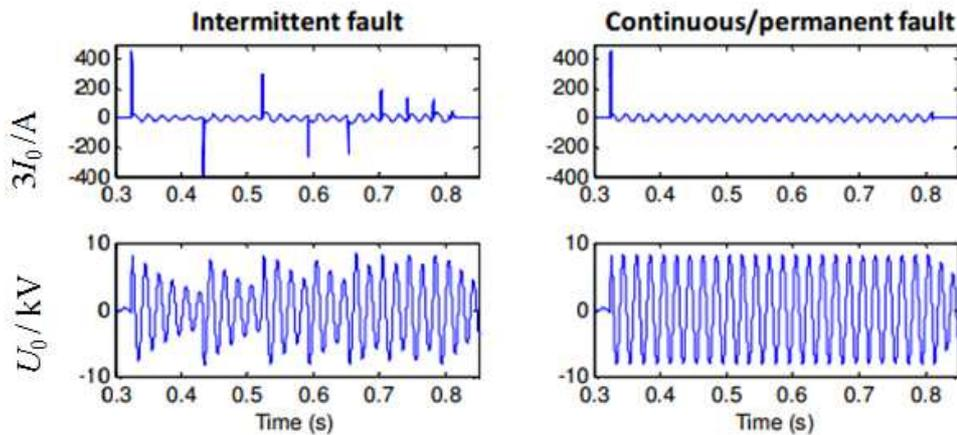
**Figure 7.** Comparison of intermittent earth fault waveforms and permanent earth fault waveforms. (Wahlroos et al. 2011.)
