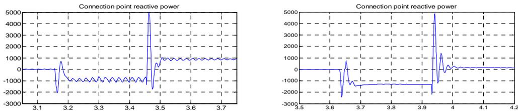
Fig. 5. Connection point reactive power: a) Without transient flux compensation, b) with the compensation.
