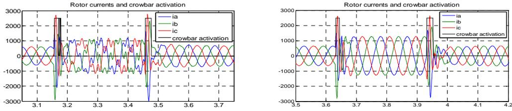
Fig. 3. Rotor currents and crowbar activation: a) Without transient flux compensation, b) with the compensation.
