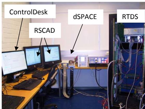
Fig. 2. The hardware arrangement of the real-time simulation environment.
