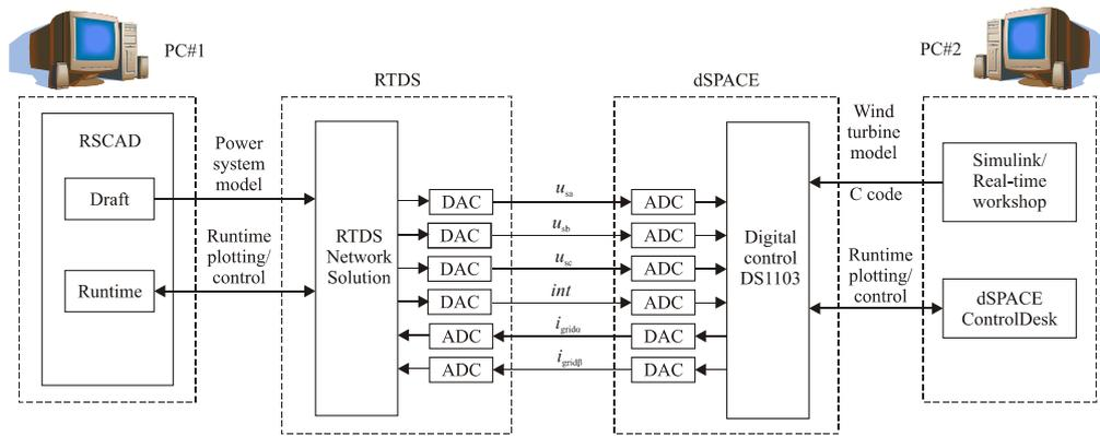
Fig. 1. Block diagram of the RTDS/dSPACE implementation.
