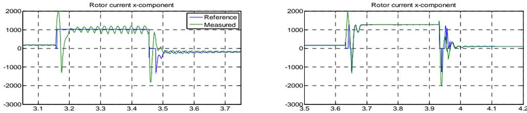
Fig. 4. Rotor reactive current component: a) Without transient flux compensation, b) with the compensation.
