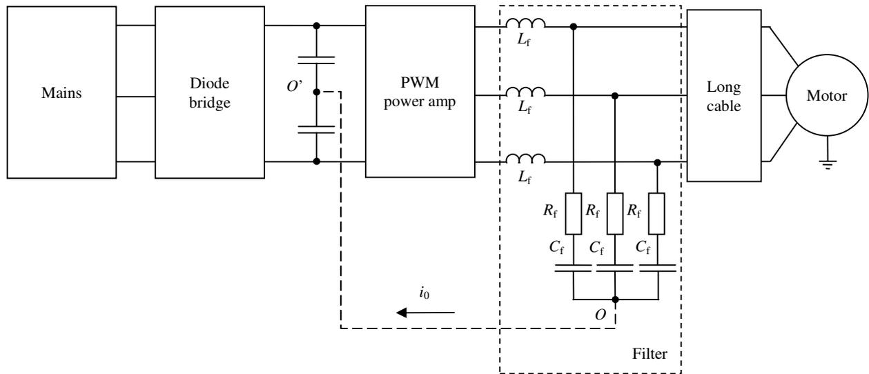
Fig. 1. A typical converter-based electrical drive topology with filter.
