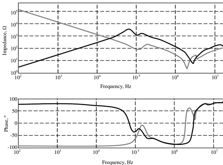
Fig. 2. Differential-mode (—) and common-mode (---), impedances of the Strömberg three-phase 22 kW induction motor used in the test setup.
