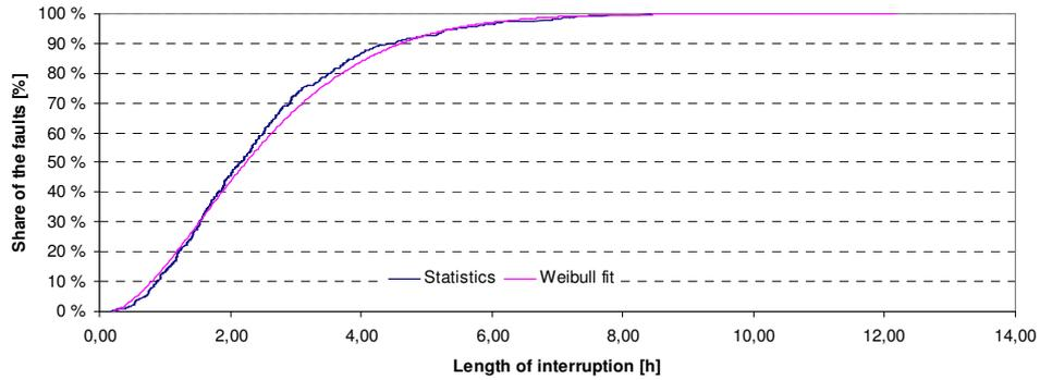
*Figure 5 An example distribution of fault durations, which consists of 487 separate interruptions.*
