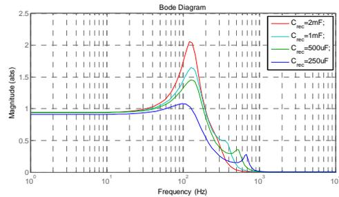
Figure 3. System frequency response. Rectifier capacitance is varied; Inverter capacitance is fixed at 1600 $\mu\text{F}$ .
