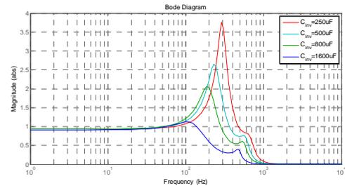
Figure 2. System frequency response. Inverter DC capacitance is varied; Rectifier DC capacitance is fixed at 500 $\mu\text{F}$ .
