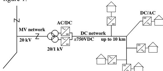
**Figure 1. Basic concept of LVDC distribution network**
