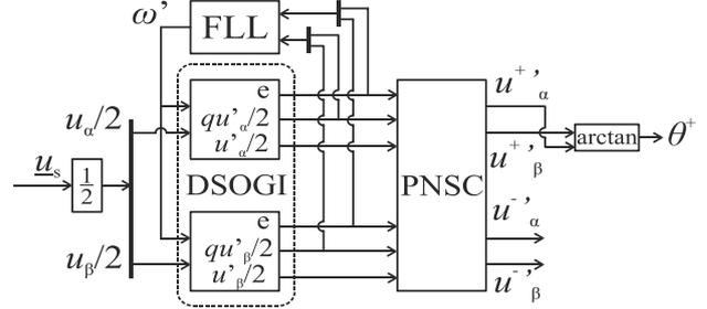
Fig. 7 Schematic diagram of DSOGI-FLL [13].
