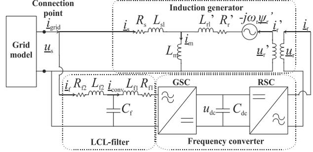
Fig. 5 Equivalent circuit of the DFIG
