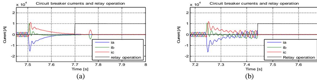
Fig. 14 CB current and relay operation: (a) without reactive current injection; (b) with reactive current injection.
