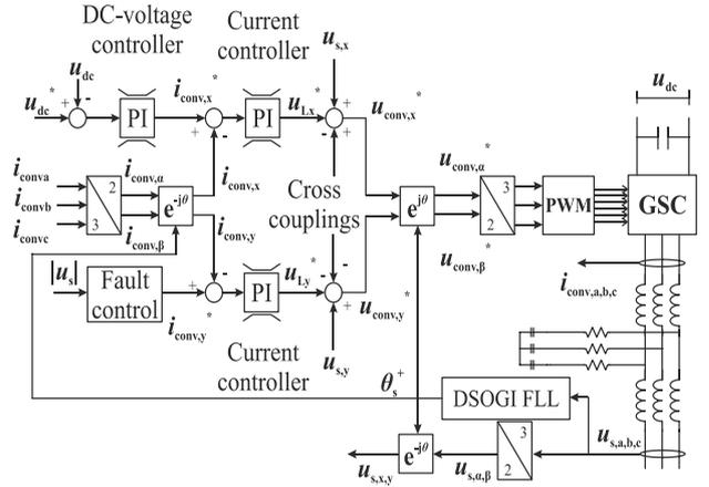
Fig. 8 Control of grid side converter.
