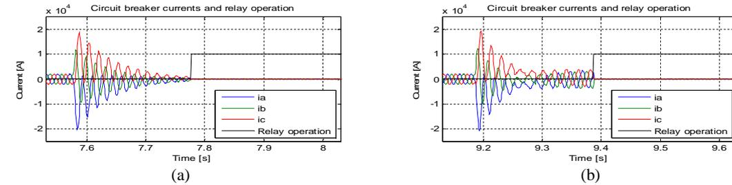
Fig. 17 CB current and relay operation: (a) without reactive current injection; (b) with reactive current injection.
