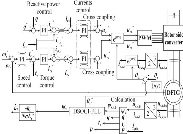
**Fig. 9 Control of rotor side converter.**
