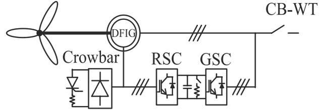
**Fig. 3** DFIG with passive crowbar protection [4].
