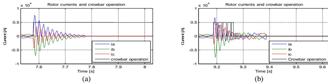
Fig. 16 Rotor current and crowbar operation: (a) without reactive current injection; (b) with reactive current injection.
