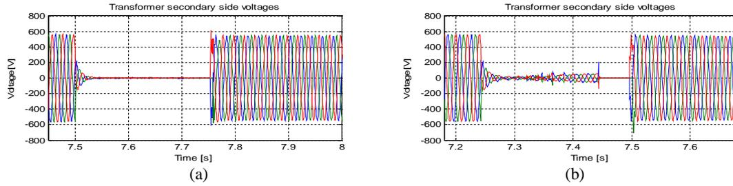
Fig. 12 Connection point voltage: (a) without reactive current injection; (b) with reactive current injection.
