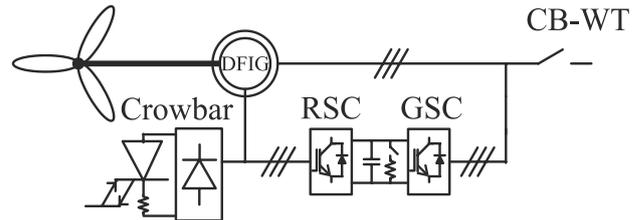
**Fig. 4** DFIG with active crowbar protection.
