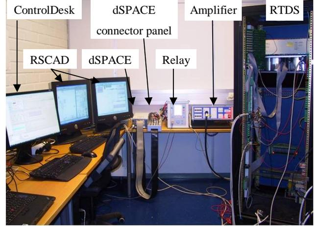
Fig. 10 Hardware-in-the-loop test setup.
