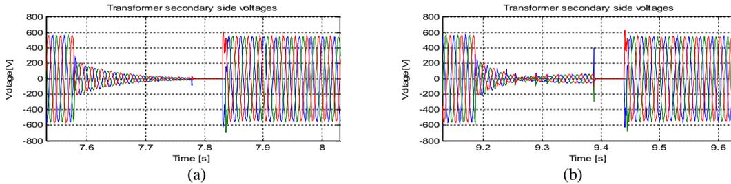
Fig. 15 Connection point voltage: (a) without reactive current injection, (b) with reactive current injection.
