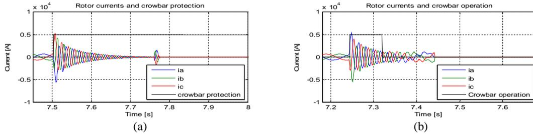
Fig. 13 Rotor current and crowbar operation: (a) without reactive current injection; (b) with reactive current injection.
