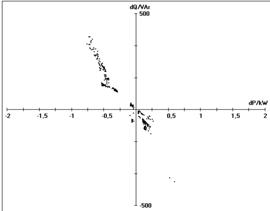
Fig. 20. Average power signatures of an inverter based air source heat pump.
