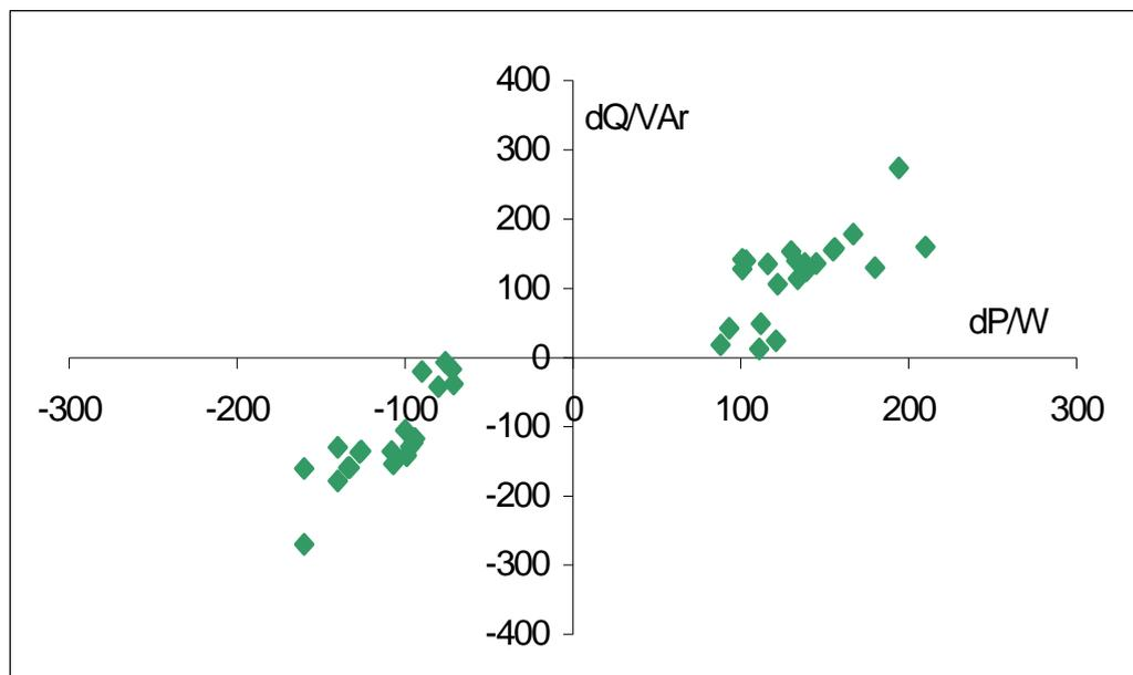
Fig 9. Average power signatures of twenty different domestic refrigeration appliances.
