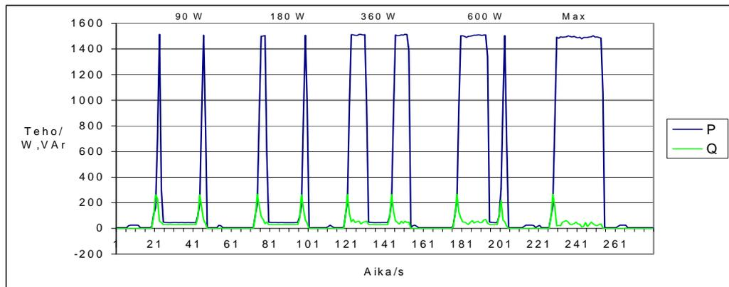
Fig. 14 Load curve of a microwave oven at different power level.
