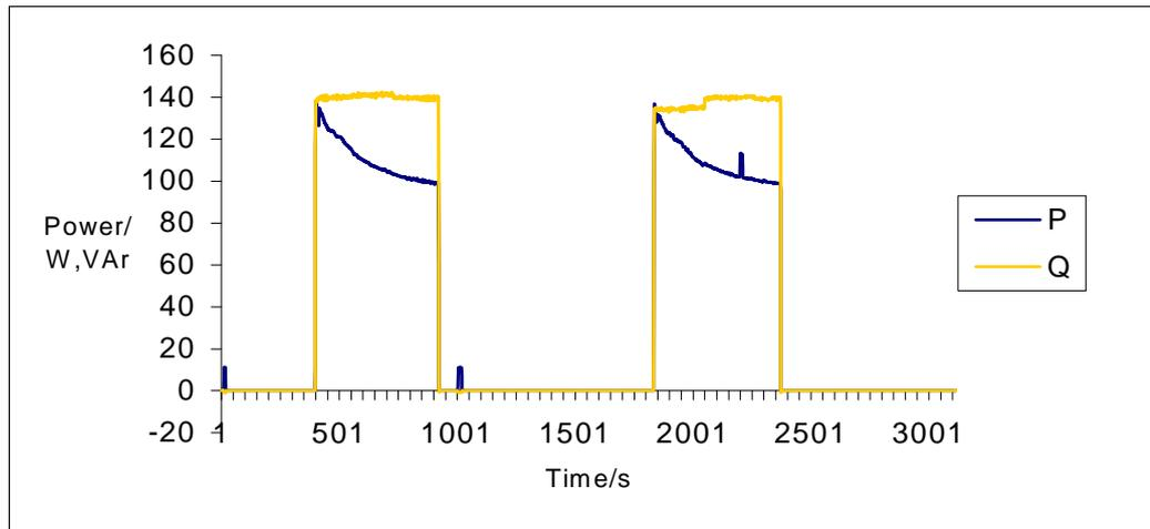
Fig 8. Cooling compressor cycles of a refrigerator ( $P$  active power,  $Q$  reactive power).
