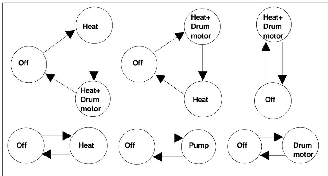
Fig. 7. Model of a typical clothes washer (Pihala 1998).
