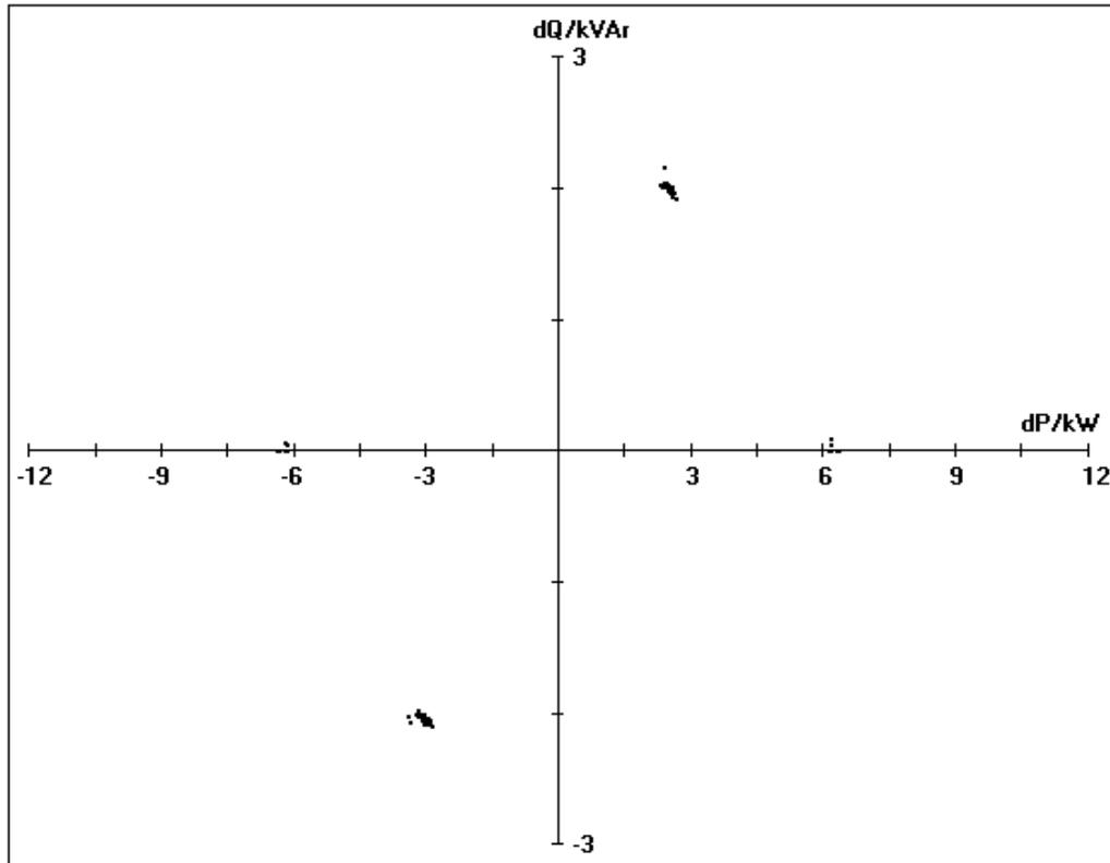
Fig. 17. The average three-phase power signatures of a geothermal heat pump compressor and the extra heater.
