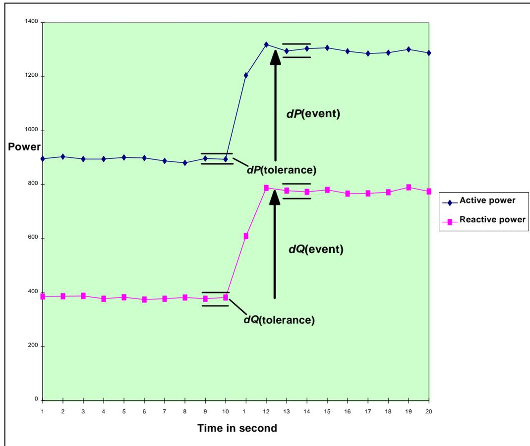
Fig. 2. Detecting an event in sample data caused by an appliance (Pihala 1998).
