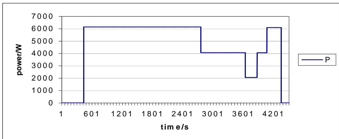
Fig. 22. An example of load curve of a sauna stove controlled by a multistate thermostat.
