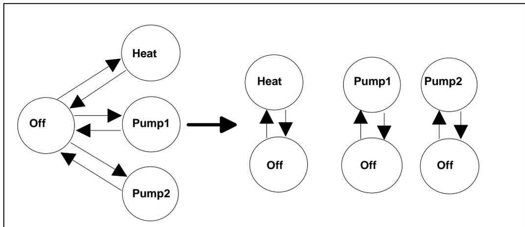
Fig. 6. Breaking a model of a dishwasher into many two-state models.
