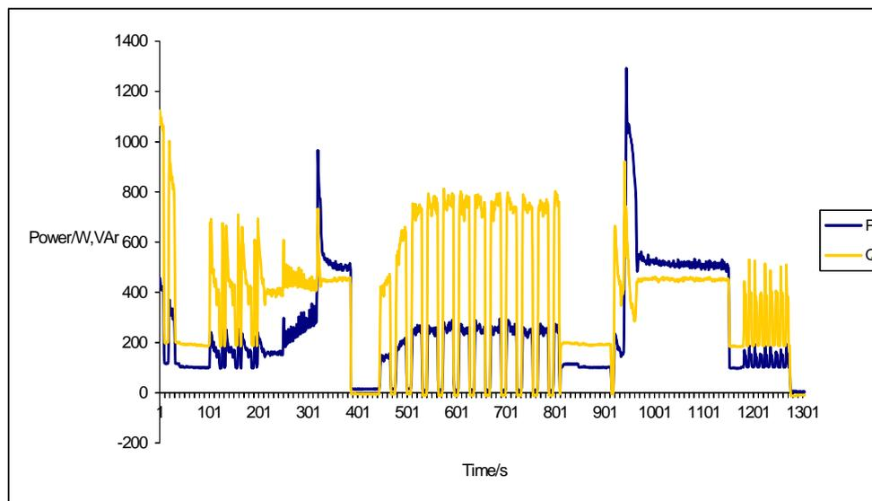
Fig. 12 Load curves of a clothes washer in last period (spin-dry).
