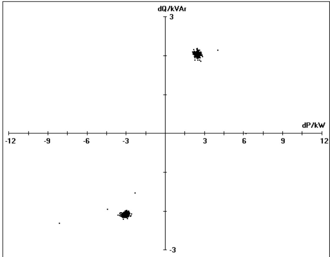
Fig. 18. Average three-phase power signatures of a geothermal heat pump compressor during two months in the spring.
