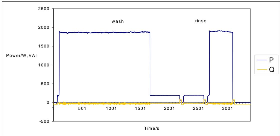
Fig. 10 Typical load curve of a dishwasher ( $P$  active and  $Q$  reactive power).
