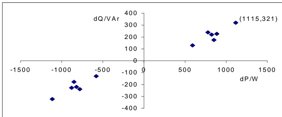
Fig. 16 Average power signatures of six vacuum cleaners.
