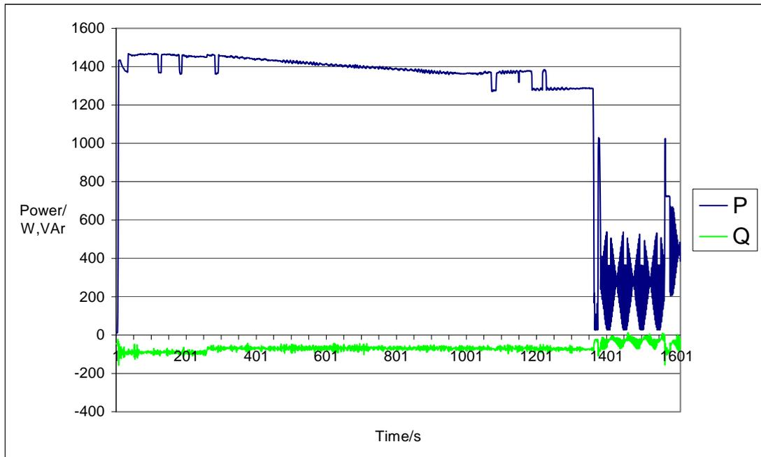
Fig. 21. An example of a load curve of inductive heating of water in a kettle.
