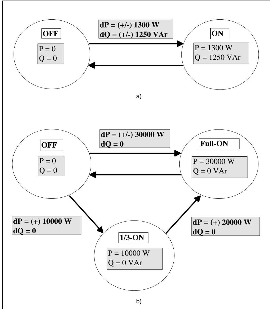
Fig. 5. Finite-state appliance models: a) generic two-state appliance, water pump b) multi-state appliance, hot water boiler (Pihala 1998).
