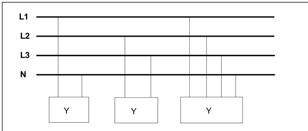
Fig. 4. Different possibilities to wire appliances ( $Y$ ) on power lines in a three phase system ( $L+N$ ,  $L+L$  or  $L+L+L+N$ )(Pihala 1998).
