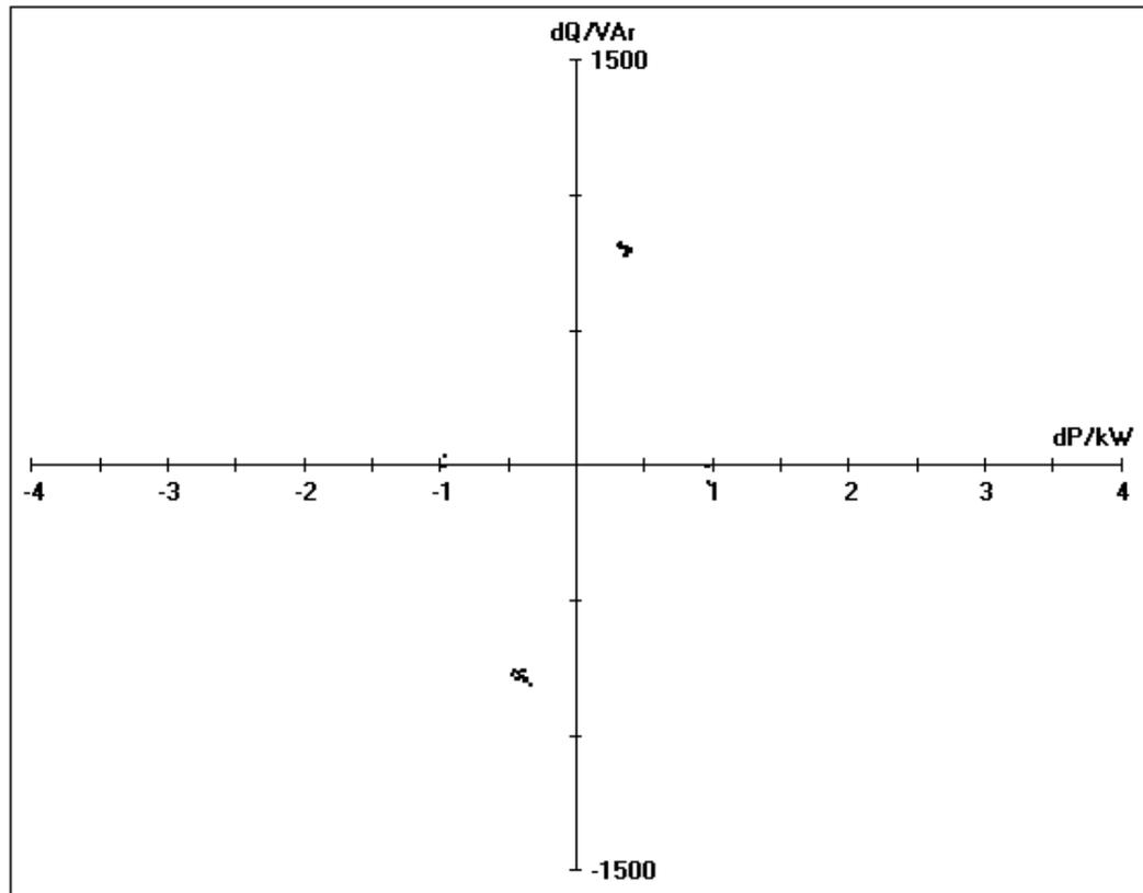
*Fig. 19. Average power signatures of an active heating recovery heat pump compressor and the extra heater.*
