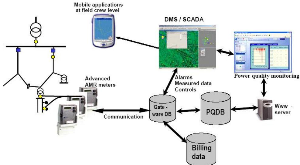
Figure 6 . The overall view of IT architecture in the pilot case
