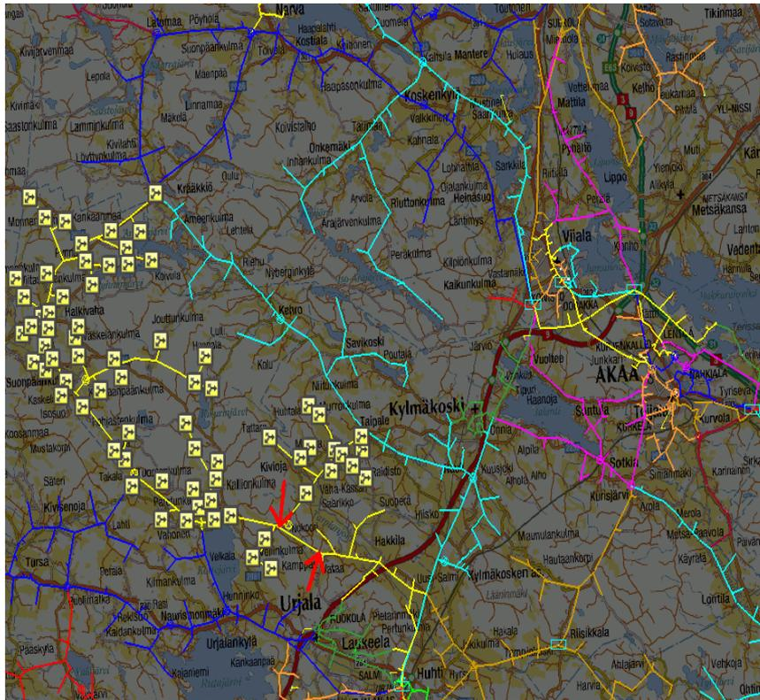
Figure 5. Broken conductor fault is located automatically.
