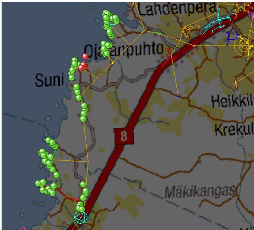
Figure 4. After MV fault is repaired remaining faults in LV network were found automatically by DMS.
