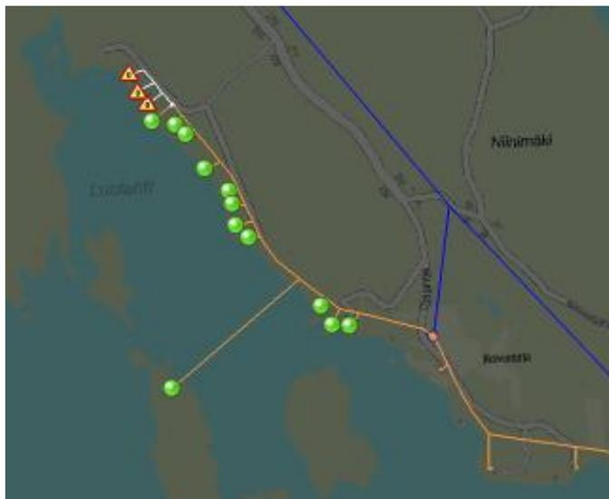
Figure 2. Three neutral fault alarms are shown by DMS.
