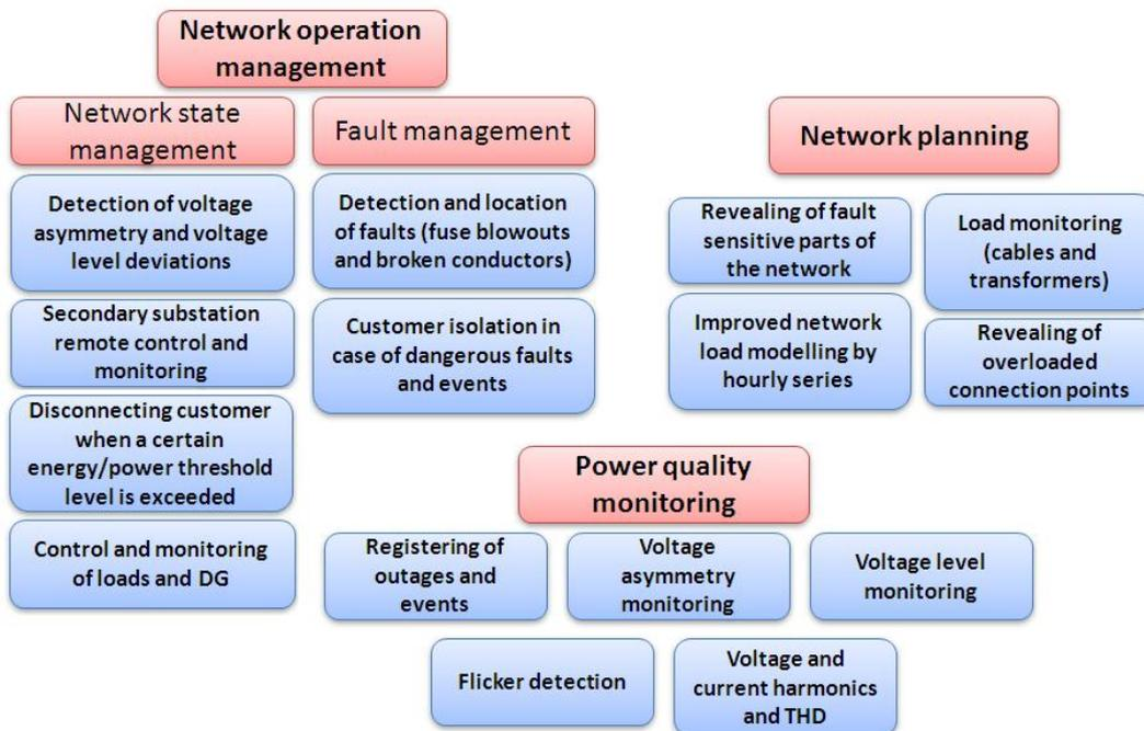
Fig. 9. Utilizing AMI in LV network management.
