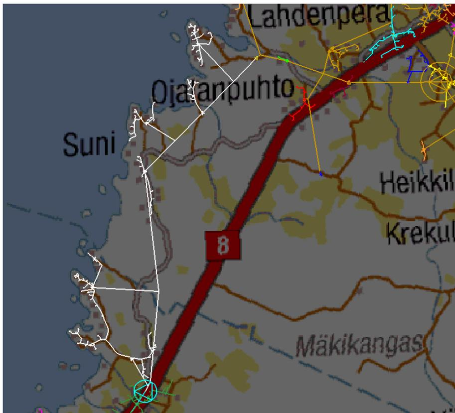
Figure 3. MV fault is just detected in DMS.
