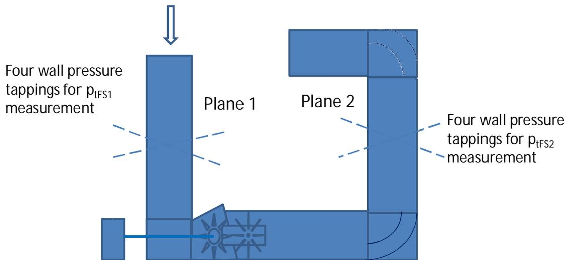
$$\begin{aligned} \text{Fan pressure :} & \quad p_{tFS1} \text{ measured} \\ p_{tFS} = p_{tFS2} - p_{tFS1} & \quad p_{tFS2} \text{ measured} \end{aligned}$$
