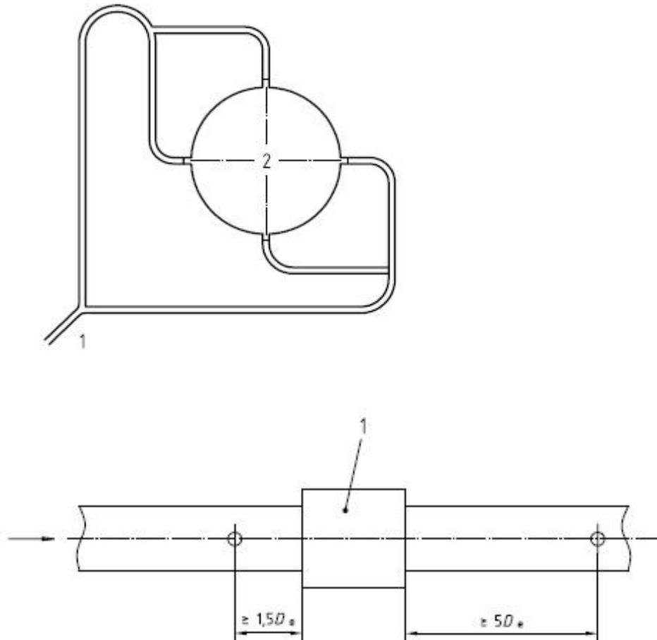
Figure 1. Upper insert: a connection of four pressure sensors for the measurement of the average pressure. Lower insert: the requirements for the location of the pressure measurement planes from the fan according to EN ISO 5802.
