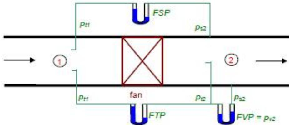
Figure 3. FTP, FSP and FVP for a fan installed in a channel /5./.
