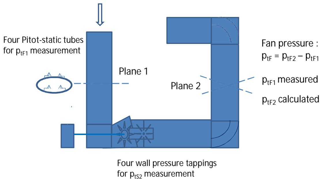
Figure 8. A combination of total pressure and static pressure measurements.
