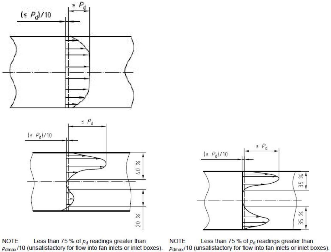
Figure 2. Upper insert: an ideal pressure distribution on the measurement plane. Lower insert: two examples of non-ideal pressure distribution.
