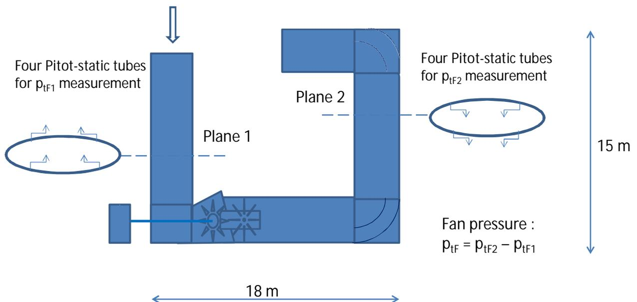
Figure 7.  $p_{tF}$  –measurements with Pitot tubes in stack.
