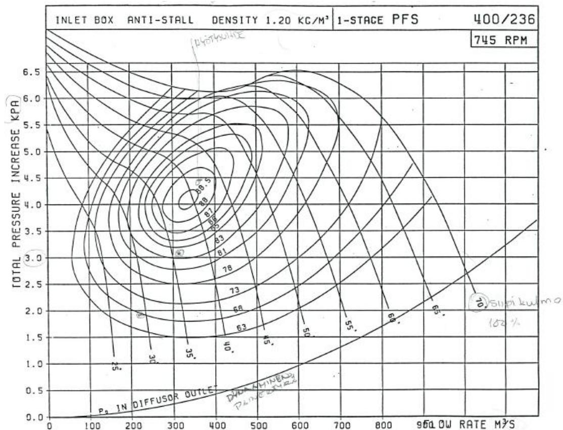
Figure 6. The fan characteristics of PFS-400-236 axial fan.
