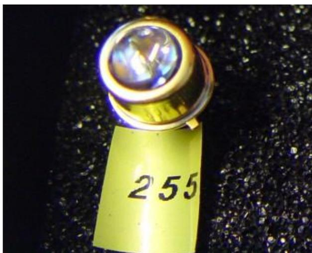
*Figure 3. SET Inc UVTOP 255 nm LED. TO39-packaged with hemispherical lens.*
