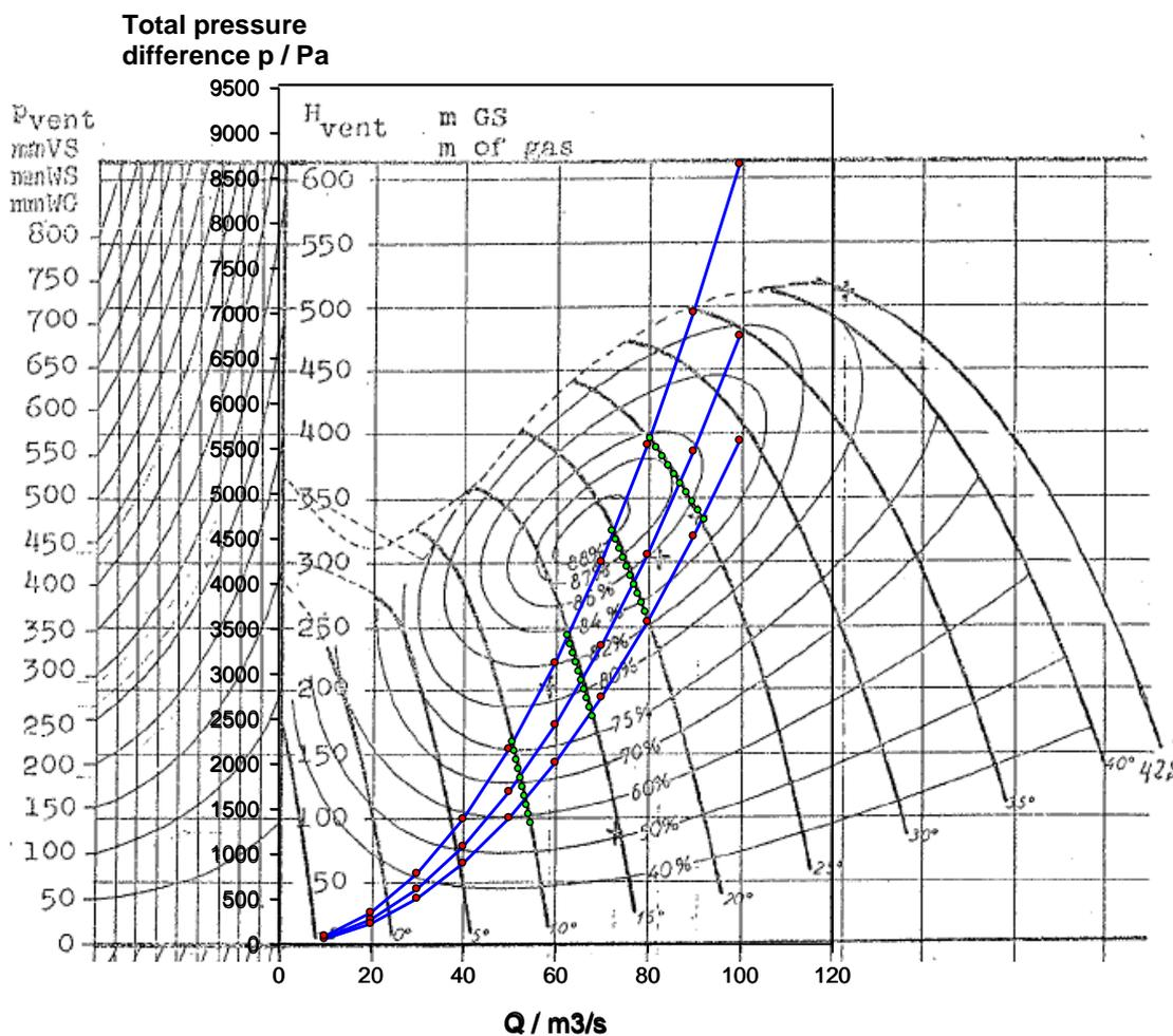
The generality of this result can be improved by checking the situation with other axial-fans. However, it seems to be difficult to obtain exact information on fan curves in digital form. Moreover, the manufacturer has not provided any uncertainty estimates to the fan curves.
