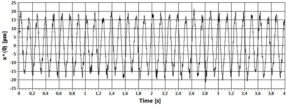
**Figure 10. Displacement signal  $x^{(0)}$  obtained from the noisy acceleration.**
