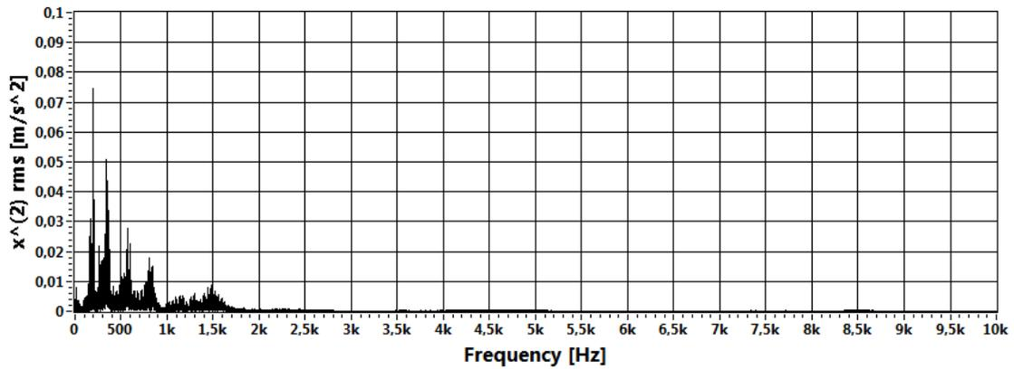
(b) The rms amplitude spectrum.
