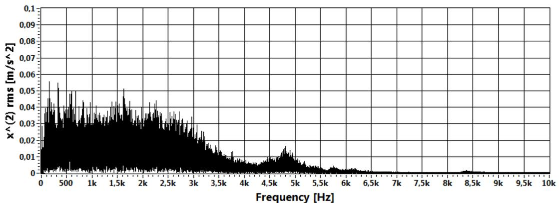
**Figure 7. The rms amplitude spectrum of the noisy acceleration signal of the faulty case.**
