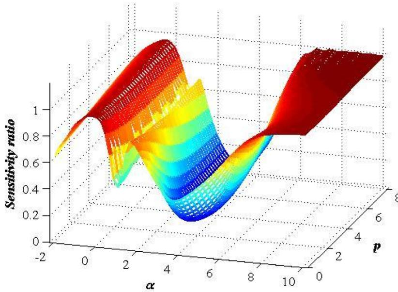
**Figure 19. Sensitivity ratio of the noisy and the original signals for generalised norms  $\|{}^\tau M_\alpha^p\|_p$ .**
