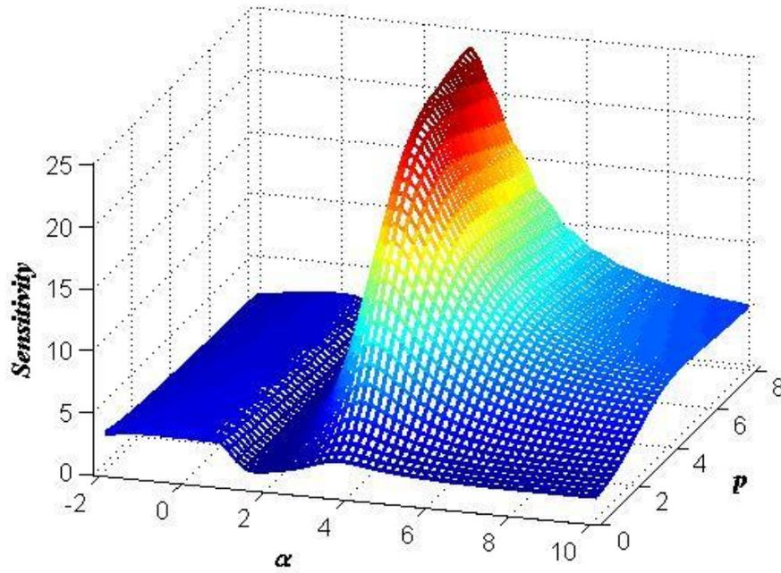
**Figure 12. Sensitivity of norms obtained from the signals in the faulty case without additional noise.**
