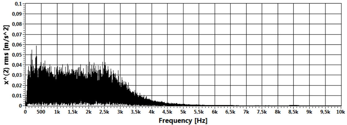
**Figure 5. The rms amplitude spectrum of the noisy acceleration signal of the intact case.**
